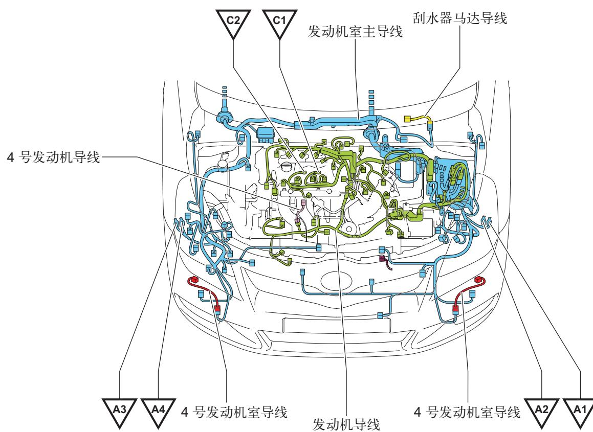
**G 布线图****□：连接线束和线束的连接器位置**
